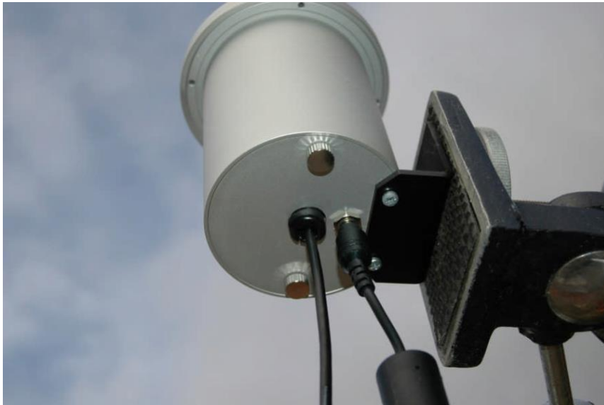
A rear view of the Oculus, showing the heater socket and USB cable.
